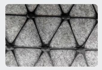
Inclusion of Ace Foundation Grid provides ground stabilisation when installed beneath the granular sub-base. Its unique triangular design dissipates loads more effectively than traditional square-shaped grids. The Ace Foundation Grid incorporates a geotextile layer to prevent soil migration, allowing for installation on otherwise unsuitable sub-grade such as clay and silt.
